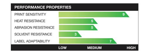
10" per second, at low print head energy, this wax maintains excellent quality on low cost substrates. This wax also has the additional advantage of being ISEGA approved for use when the printed image comes in contact with non-fatty
